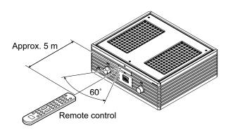
Operate the remote control within approx. 5 m distance from the front panel of the main unit within an angle of 60° to the remote sensor.
