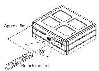
Operate the remote control within approx. 5 m distance from the front panel of the main unit within an angle of 60° to the remote sensor.
